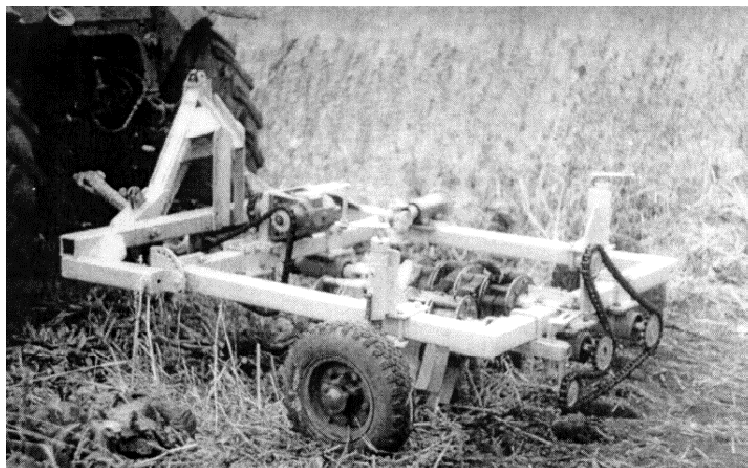
Fig. 1. General view of the experimental installation for studying cleaning of the root crop heads from the remnants of tops, attached to a wheeled aggregating tractor, class 1.4
